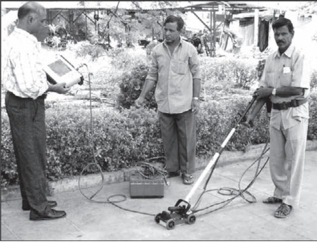
Figure 1. A typical GPR system
