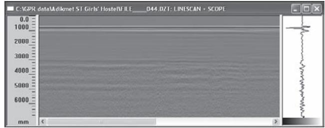
**Figure 9. Image of a soil infill with poor compaction (400 MHz antenna)**
