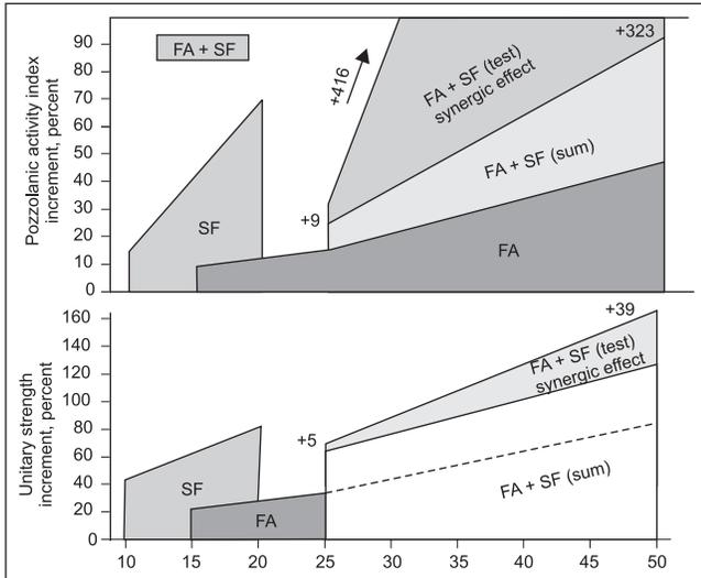
Fig 3 Synergistic effect of silica fume (SF) and fly ash (FA) on OPC<sup>20</sup>
