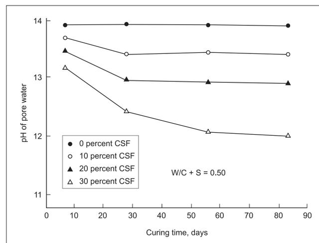
Fig 2 Effect of silica fume on the pH value of pore water solution<sup>4</sup>
