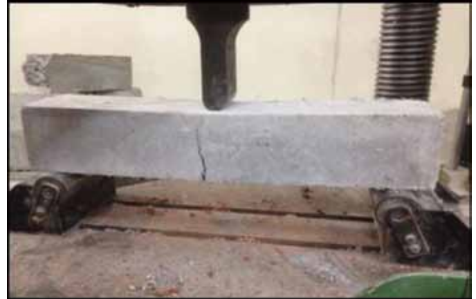
Figure 5. Flexural strength test on specimen
