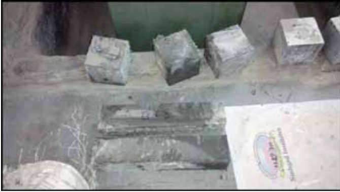
Figure 3. Specimens for compressive and flexural test
