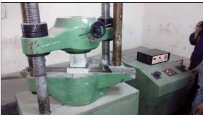
Figure 4. Compressive strength test on specimen
