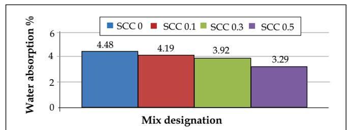
Figure 6. Results of water absorption for various mixes
