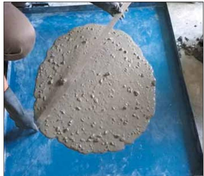
Figure 2. Slump flow test for SCC
