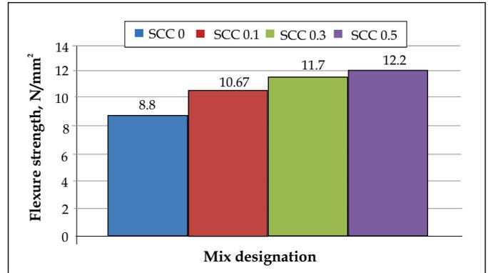
Figure 5. Results of flexural strength for various mixes
