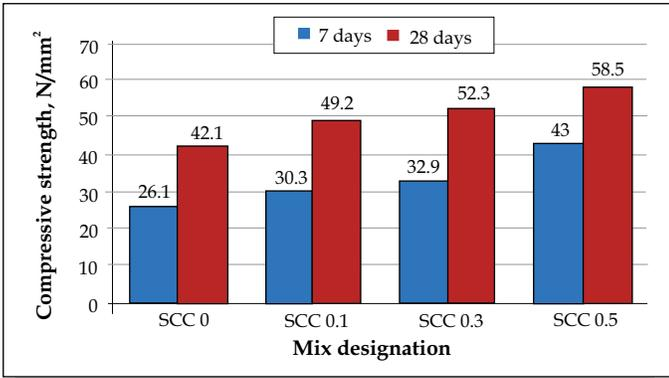
Figure 3. Results of compressive strength for various mixes
