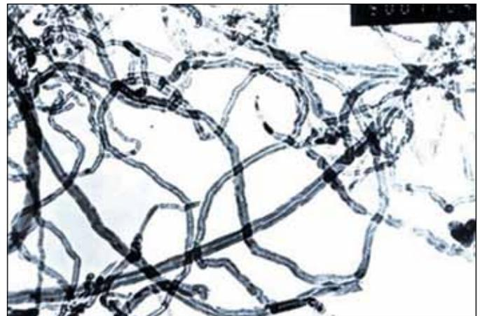
Figure 1. TEM image of multi walled carbon nano tubes
