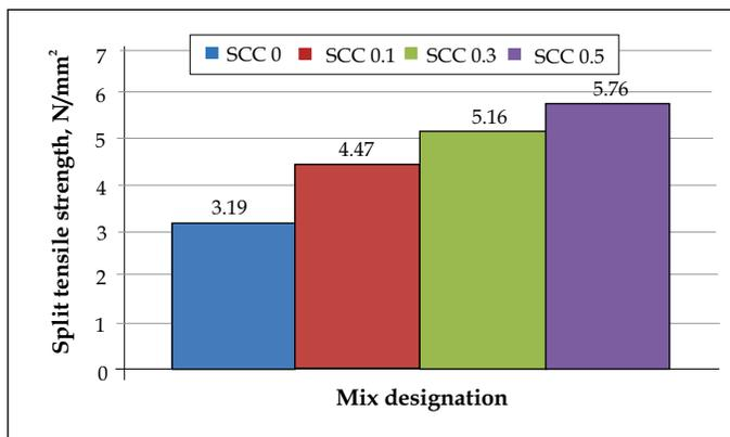
Figure 4. Results of split tensile strength for various mixes
