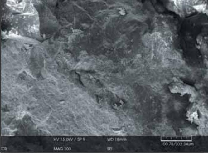
Figure 7. SEM Image of concrete with nano tube
