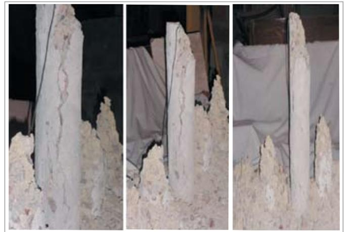
Figure 3. Failure in columns without confinement after single heating-cooling cycle at elevated temperatures
