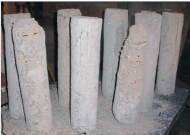
Figure 5. Spalling in columns confined with steel reinforcement at elevated temperature
