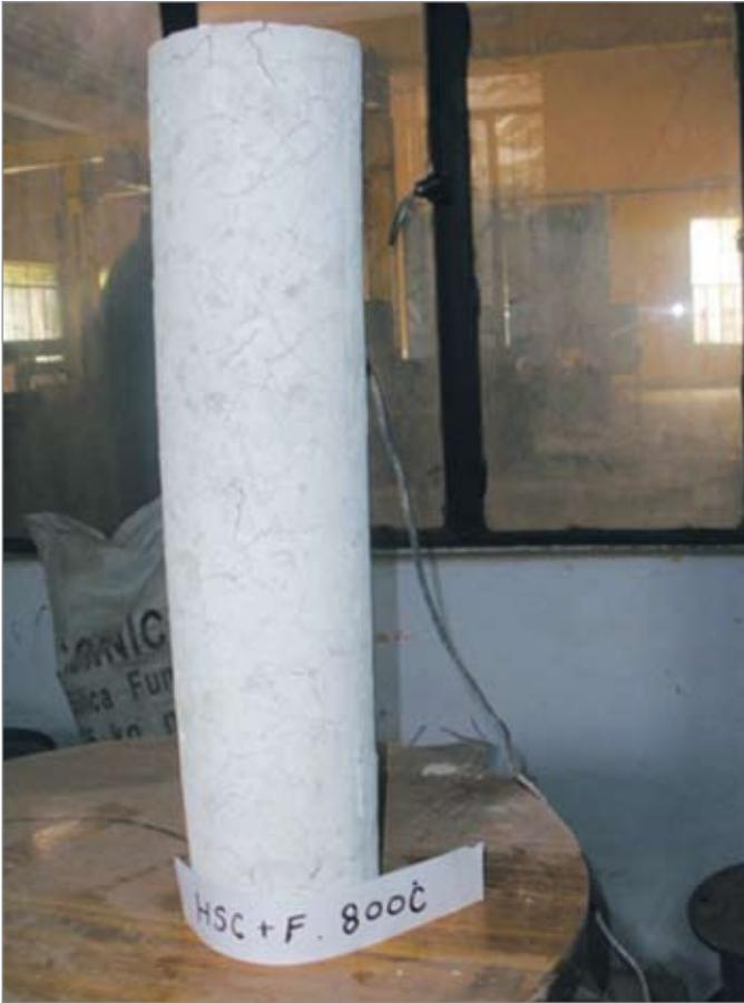
Figure 4. Confined column with fibers with extensive cracks before spalling at 800°C
