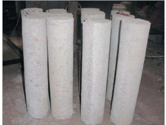
Figure 6. Behavior of columns confined with fibers and steel reinforcement after single heating-cooling cycle at elevated temperature
