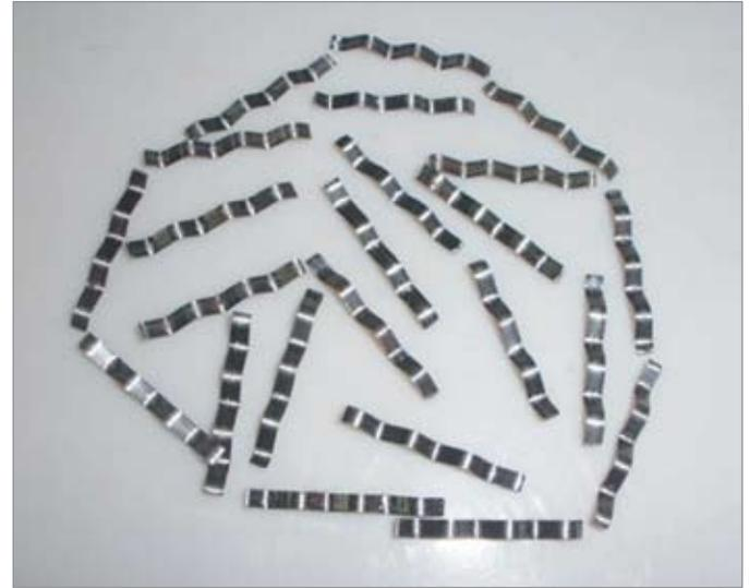
Figure 1. Crimped carbon steel fiber with crescent shaped cross section
