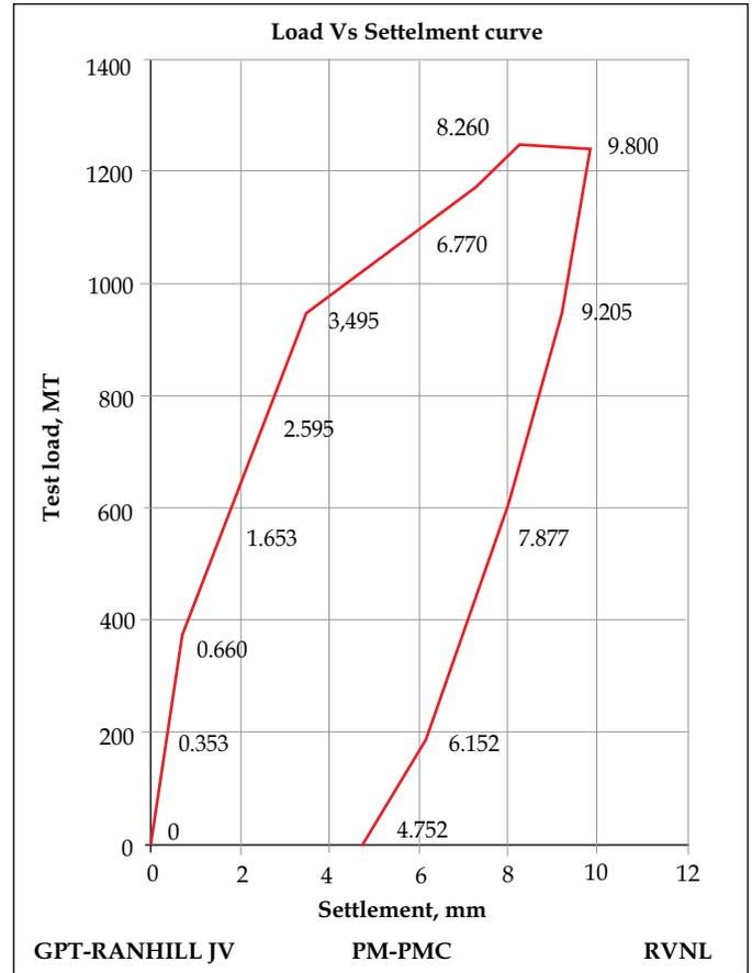
Figure 4. Routine vertical load test at pylon location
