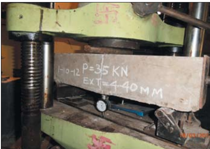
Figure 6. Measurement of deflections for PSC beam C1
