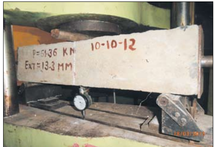
Figure 9. Measurement of deflections for PSC beam C2
