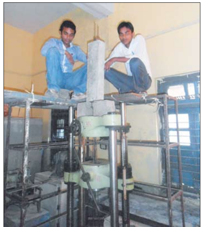
Figure 3. Vertical oriented beam for prestressing by UTM
