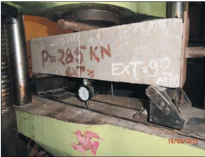
Figure 5. Measurement of deflections for PSC beam B1
