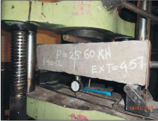
Figure 4. Measurement of deflections for PSC beam A1
