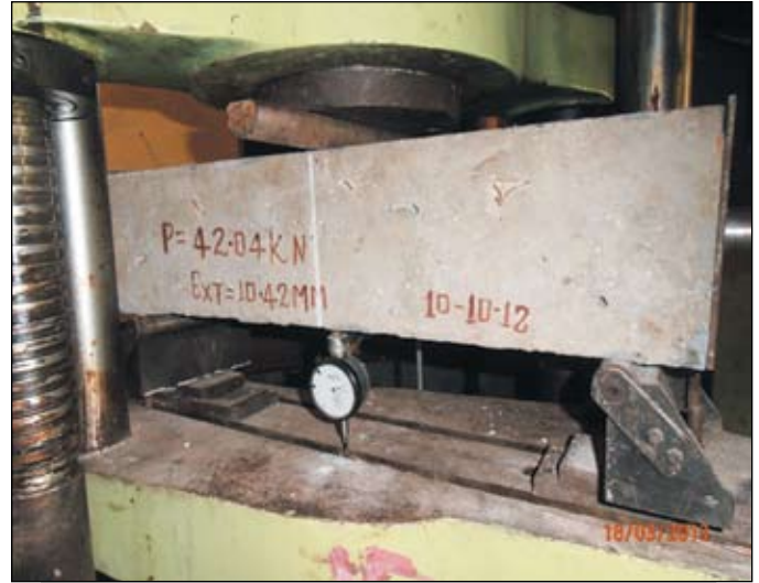
Figure 7. Measurement of deflections for PSC beam A2
