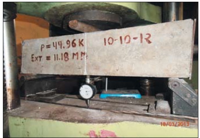
Figure 8. Measurement of deflections for PSC beam B2
