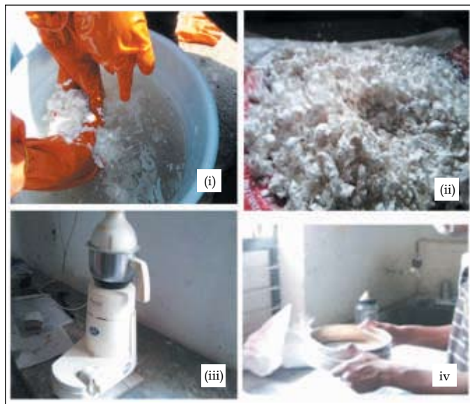
Figure 1. Processing of eggshell waste (i) washing, (ii) air drying, (iii) grinding and (iv) sieving
