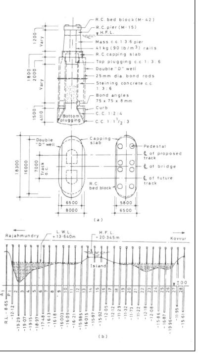
Figure 1. (a) A typical cross section of the pier showing well foundation and plan of pier cap (b) A longitudinal section showing foundation level for piers and abutments
