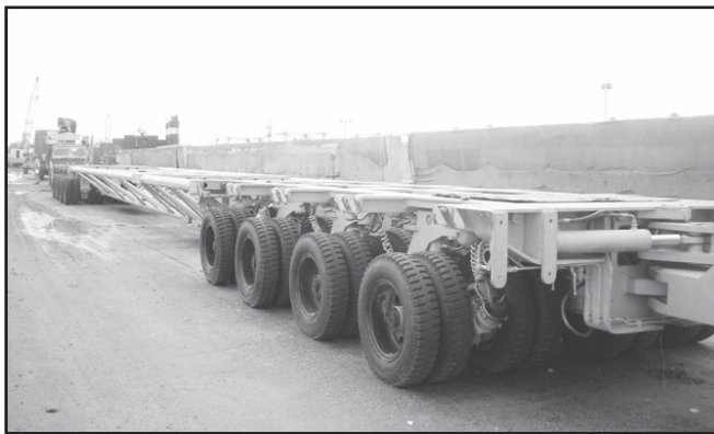
Figure 12. View of trailer for transport of full spans
