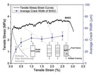
Figure 3: Typical tensile stress – strain behaviour of ECC with average crack-width data.<sup>[6]</sup>
