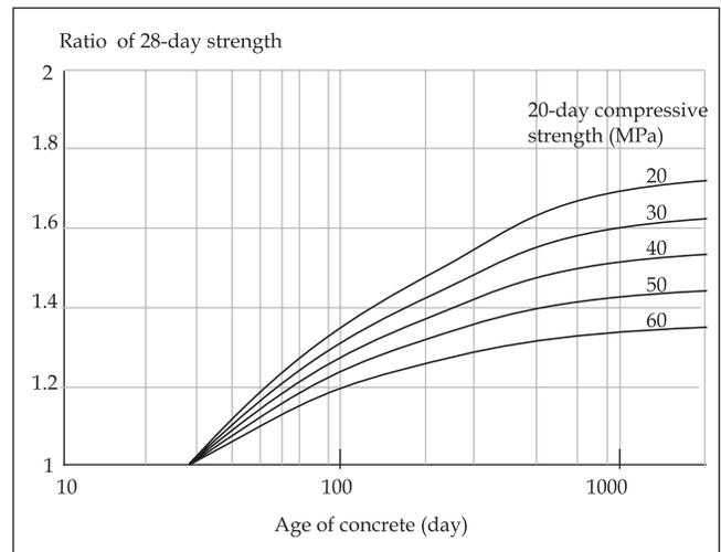
Figure 1. Relationship between age and compressive strength for pavement quality concrete<sup>2</sup>
