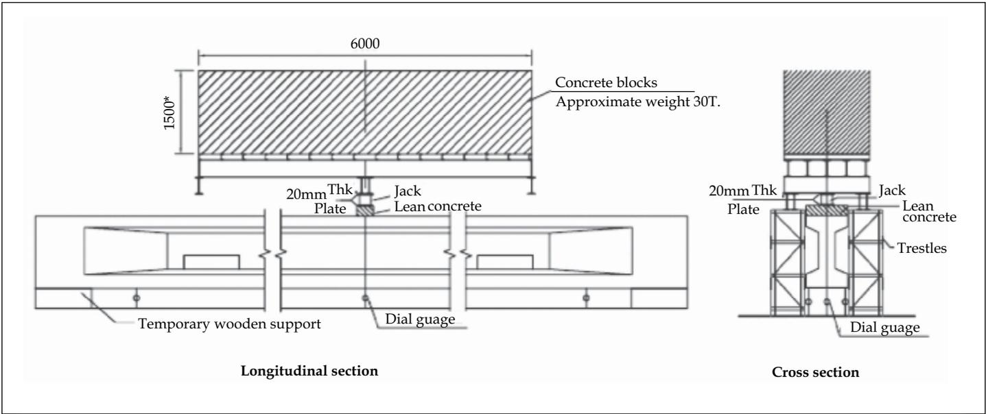
Figure 3. Girder load test
