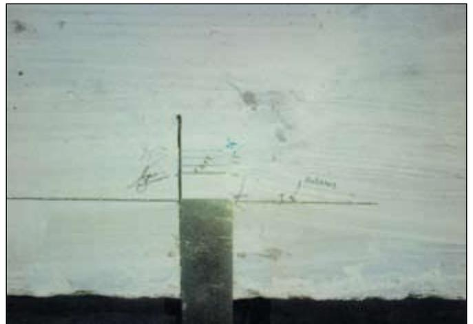
Figure 7. Residual deflection after 24 hrs of girder unloading
