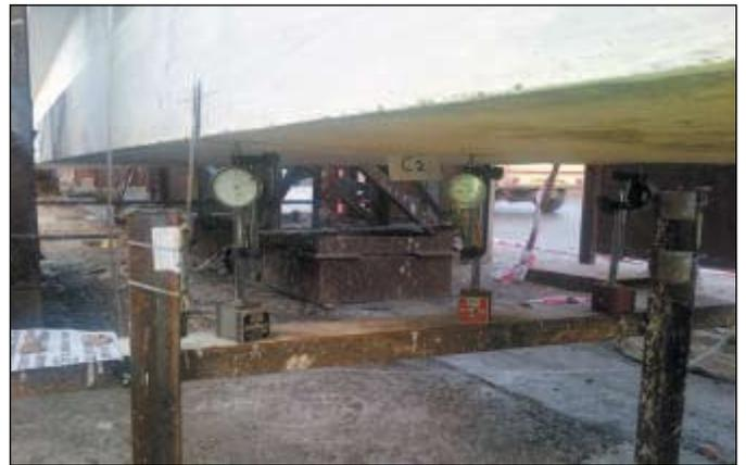
Figure 5. The measurement arrangement during girder load test
