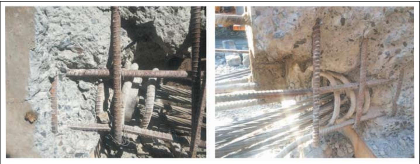
Figure 9. Cone failures
