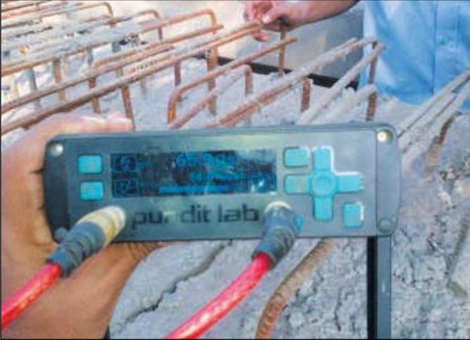
Figure 8. Combination of ultrasonic & rebound hammer test showing girder concrete strength as 54.0 N/mm<sup>2</sup>
