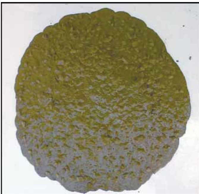
Figure 1. Slump flow test
