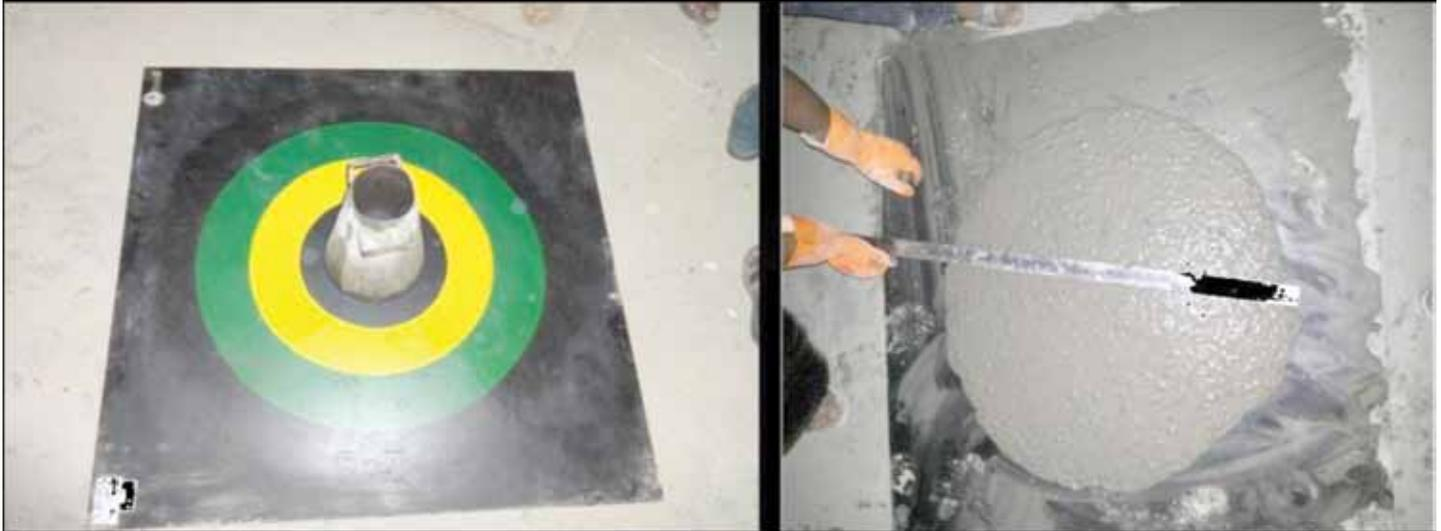
Figure 2. Slump flow test
