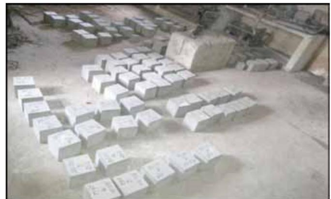
Figure 6. Concrete Specimens under self-curing
