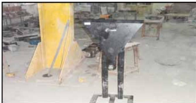
Figure 5. V funnel test
