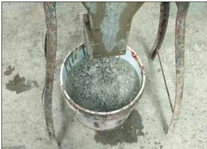
Figure 4. Mix 2 after passing through V funnel in the bucket
