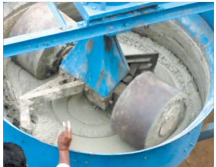
Figure 3. Roller mixer used for mixing NAC
