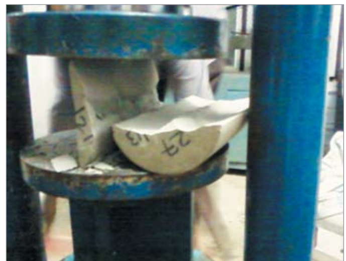
Figure 6. Split tensile testing of a NAC cylinder
