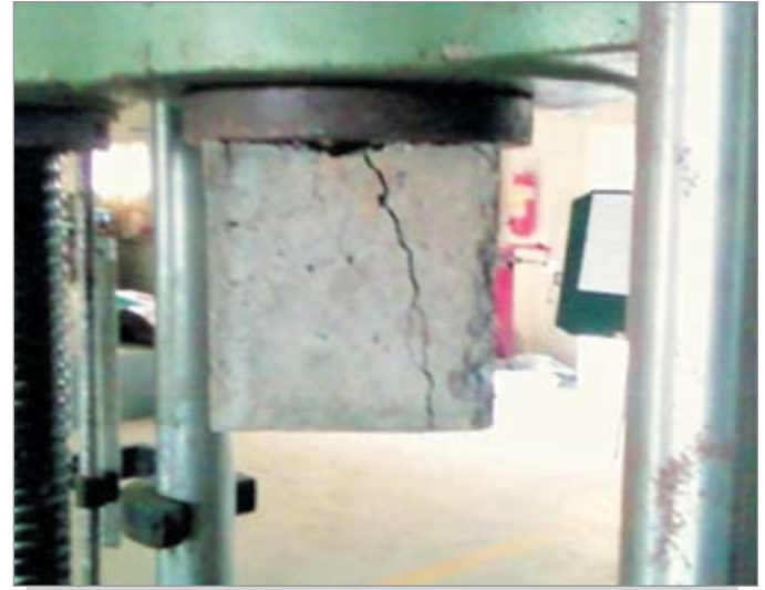
Figure 8. Bond strength testing of a 15 cm cube of control concrete
