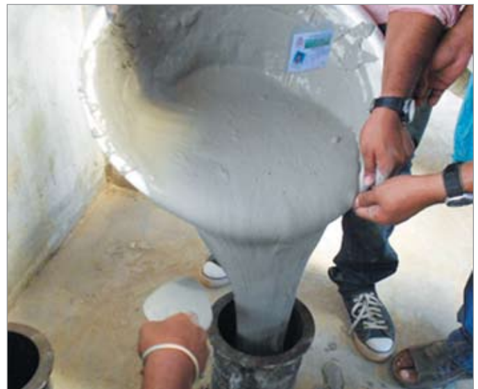
Figure 2. Casting of NAC specimen
