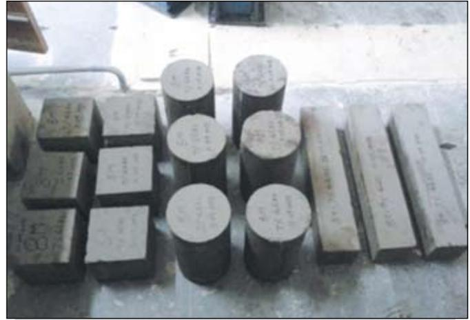
Figure 2. Demoulded cubes, cylinders and prisms
