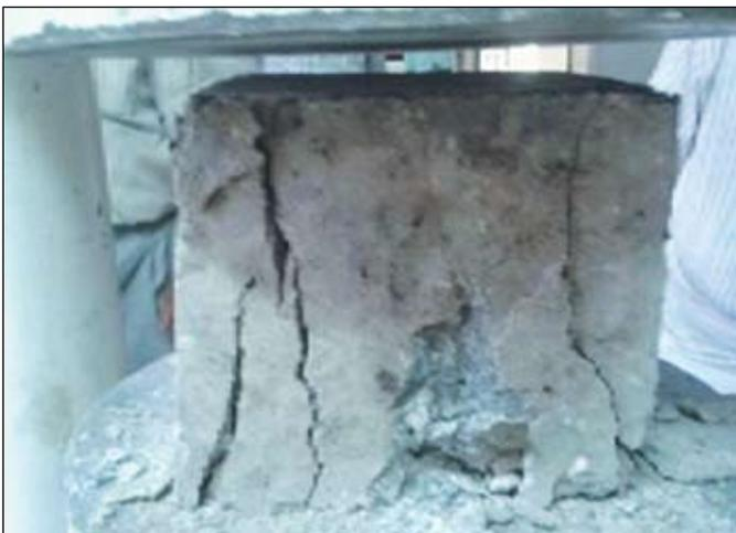
Figure 3. Failure mode of cube specimen
