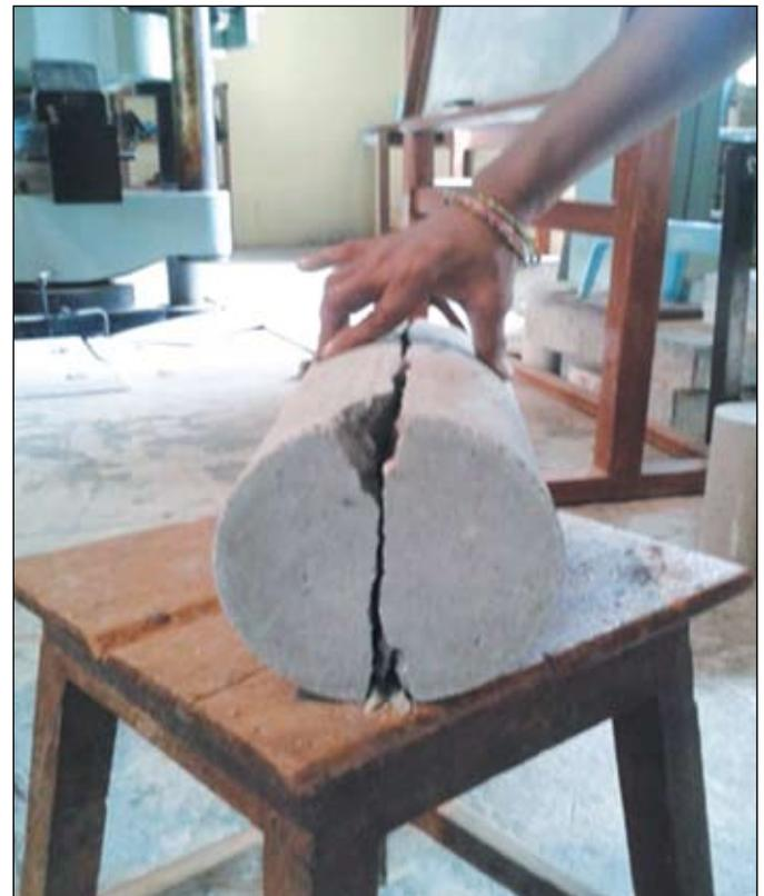
Figure 4. Tested cylinder specimen
