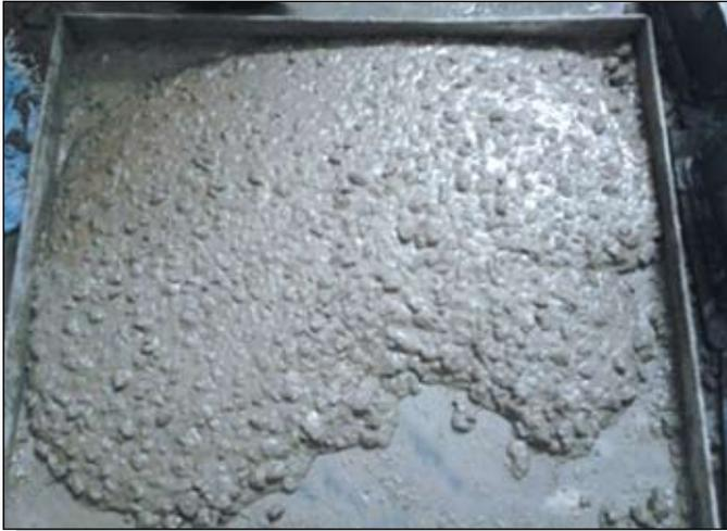
Figure 1. Freshly mixed geopolymer concrete
