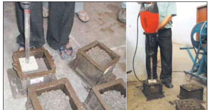
Figure 3. Compaction of DLC cubes using vibrating hammer
