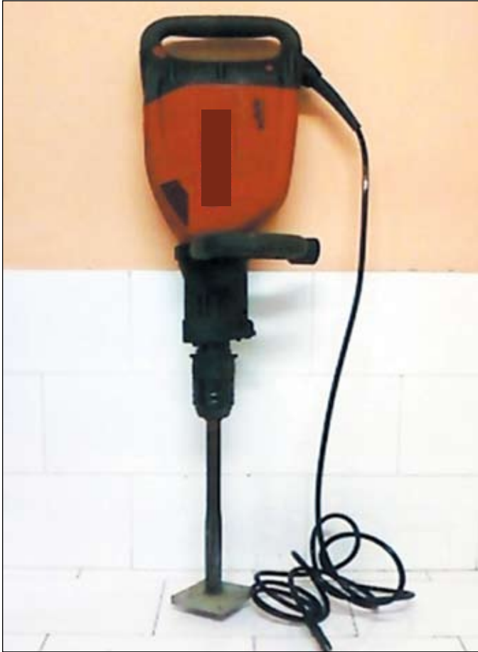
Figure 2. Vibrating hammer used for the compaction of DLC cubes
