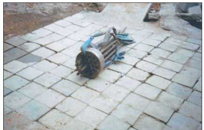
Figure 2. Poor quality of H.T. strands
