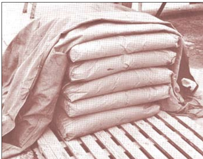
Figure 1. Storage of bagged cement ( Courtesy: Concrete practice by cement & concrete association, UK ) [10]
