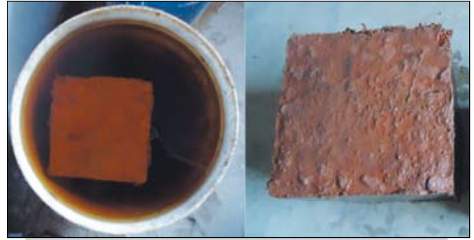
Figure 3. Water absorption test
