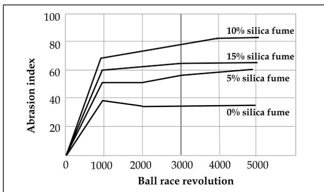
Figure 4. Abrasion index of silica fume concretes at 5 minutes testing period (Cement = 383 kg/m<sup>3</sup>; w/C+sf) = 0.32 and 28 days curing)
