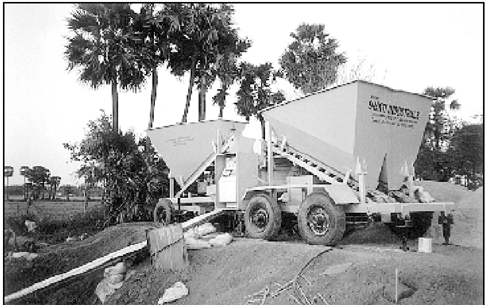
30 M supermobile concrete batching plant
