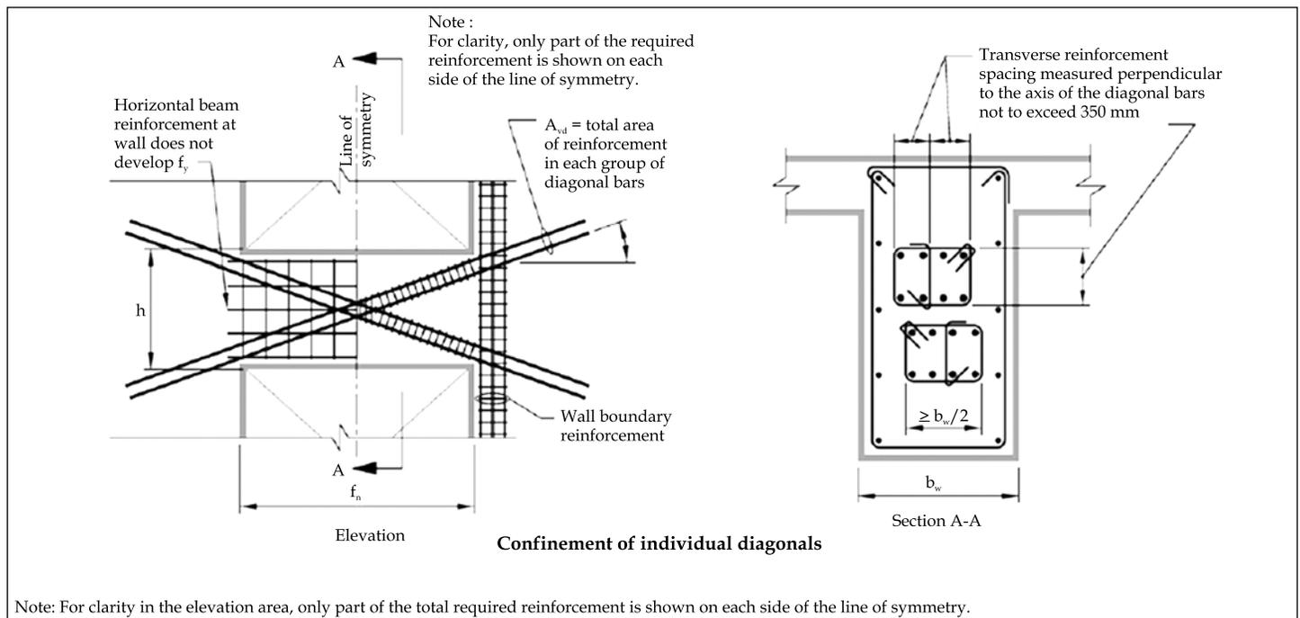
Figure 10. Coupling beams with diagonally oriented reinforcement. Wall boundary reinforcement shown on one side only for clarity (Source: ACI 318:2014)
