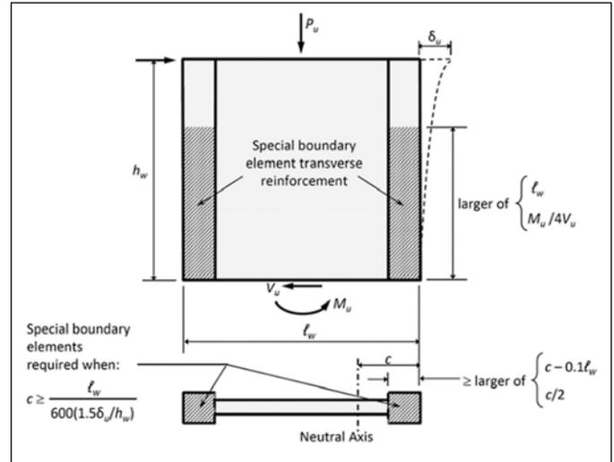
Figure 6. Specially confined boundary zone of special structural wall
