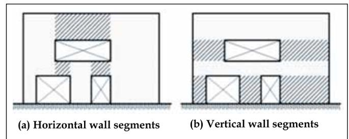
Figure 7. Wall with openings-vertical and horizontal wall segments (hatched)
