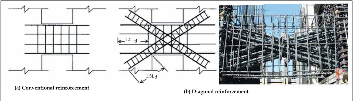
Figure 8. Diagonal reinforcement in a story-high coupling beam, an innovation introduced by Prof. Paulay and followed internationally
