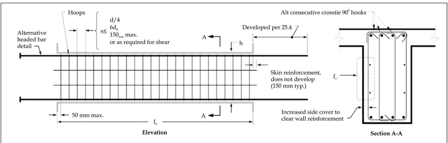
Figure 9. Details for conventionally reinforced coupling beams as per ACI 318-14 (Source: Moehle, et al. 2011)
