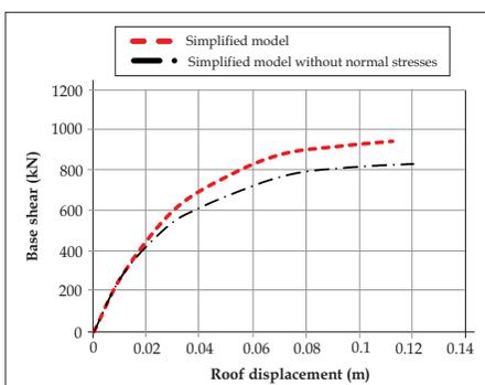
Figure 11. Comparison of pushover curves of the simplified models, with and without considering normal stresses
