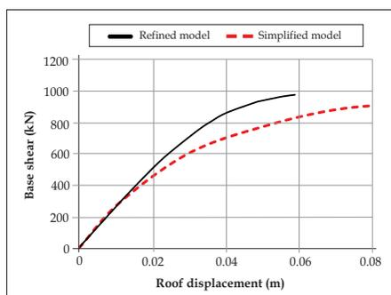
Figure 10. Comparison of pushover curves from the refined and simplified models
